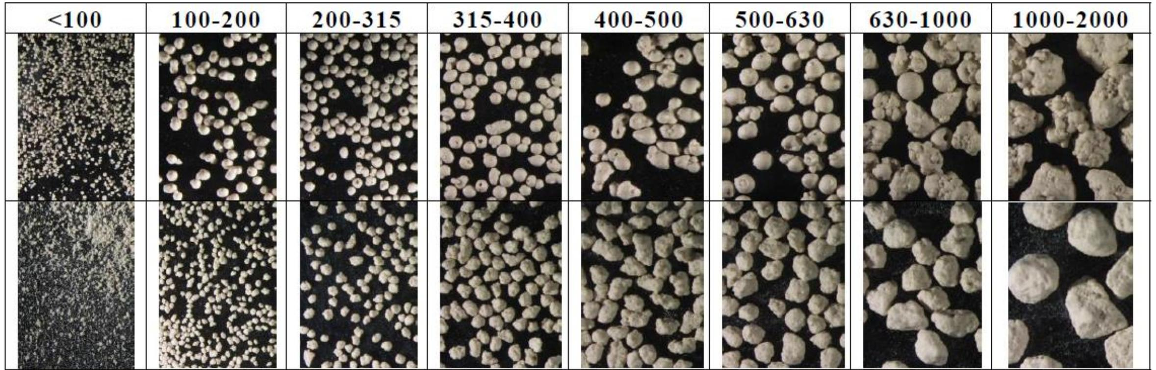
The microgranulate granules are full granules, as opposed to the spray dried granules which are “hollow”.
